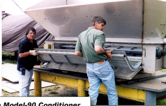
Screen Removal in a Model-90 Conditioner
