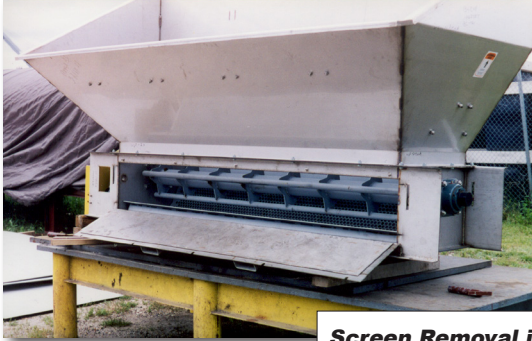
Screen Removal in a Model-90 Conditioner
