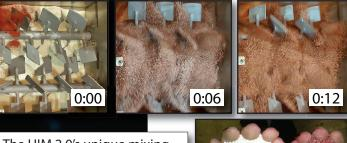
The HIM 2.0's unique mixing action ensures a homogenous blend of all types of materials from granular to powders
